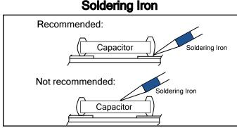
The soldering iron method is used primarily for rework or bread boarding. It is important that the solder iron tip not touch the ceramic body. The iron should be applied only to the termination-solder fillet. (Recommendation: The soldering iron shall be of the nichrome wire heater type with a maximum diameter of 3.0mm.)
